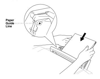
C Adjust the guides to fit the paper width.
